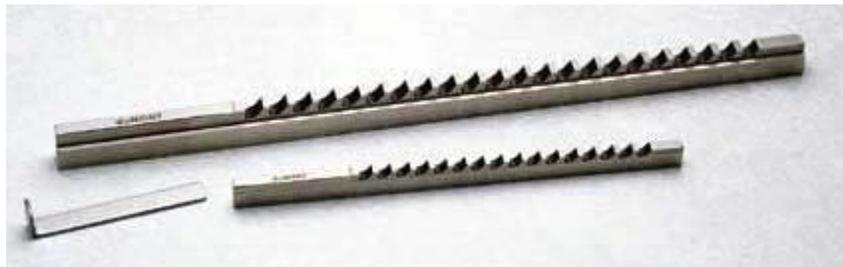
**Figure 2.** Typical push keyway broaching tools and a shim.
