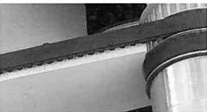
Product Ratings – Load capability of the 9 and 15mm width belts is proportional to their width. Gates belt ratings are set to guarantee long life on industrial applications. For FIRST applications, your load capability is going to be determined by the shaft to sprocket connections, belt wrap, and the ability to pretension the drive so that the belt does not jump teeth. With adequate belt wrap & proper installation tension, you will be surprised by the durability of this product!
