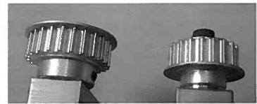
Belt Tensioning – Tension the belt so that when the drive is under full anticipated load (including shock loads) the belt does not get slack on one side, or the belt teeth try to climb out of the sprocket grooves. Make sure the mounting structure does not deflect when either tensioning the belt or under operating conditions. If you lose tension, the belt will jump teeth. Keep belt shafts parallel and sprockets in line with each other.
