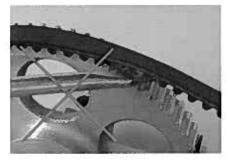
Sprocket Flanges – Provide flanges either on both sides of one sprocket or one side on the driver and the opposite side on the driven sprocket. All belts drive to one side of the sprocket. You must use flanges as described.
