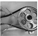
Beit Alignment - Sprockets must be aligned and shafts parallel in both planes.
