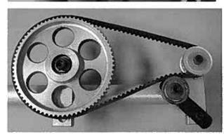
Guarding & Debris protection – A piece of flat plastic supported in between the belt spans is a simple way to eliminate pinch points and keep debris out of the drive.
