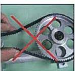
Belt Alignment – Sprockets must be aligned and shafts parallel in both planes. Alignment can easily be checked using a straight edge.
