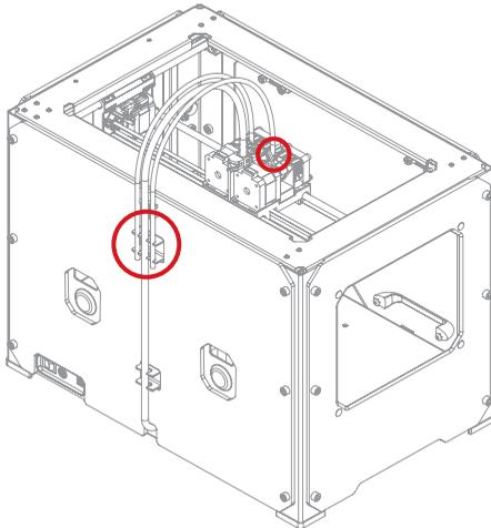
6a. Locate the two filament guide tubes. Insert one end of a filament guide tube into the hole in the top of one of the extruders. Push the filament guide tube in as far as it will go. Insert the end of the other filament guide tube into the hole on the top of the second extruder. Push the filament guide tube in as far as it will go.
