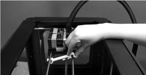
4b. A small plastic piece attached to the X-axis belt and gantry rods prevents the extruder from moving. Carefully snap the piece off of the rods and tilt it to slide it off of the belt.
