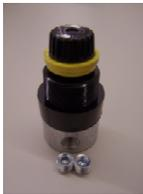
**Monnier** has donated the secondary regulator, which has a yellow ring around it. This is also a relieving regulator. Its purpose is to allow you to have a reduced pressure leg, if needed. There is an arrow denoting the direction of flow to help you identify the inlet and outlet ports. A gauge may be placed in either of the other ports and you will have to plug the other gauge port with the plugs included in the Monnier bag.
