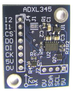
The 3-Axis Accelerometer measures both dynamic acceleration (vibration) and static acceleration (gravity). Accelerometers are sensitive to rough handling. Please remember to handle with care.
