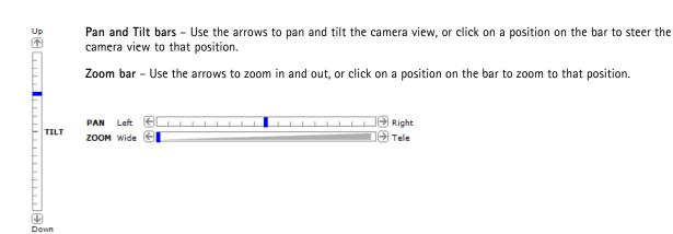
The PTZ controls can be disabled under PTZ > Advanced > Controls, see Controls, on page 23.
