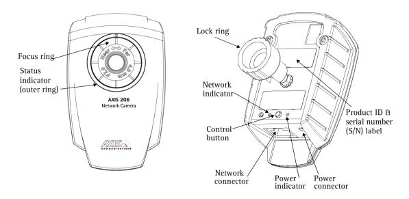
Power Connector - For connection of the PS-L power adapter (included).
