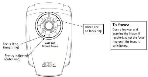
**Note:** Upon delivery, the raised line on the focus ring is aligned with the dot above the lens, and the focus is set to infinity.
