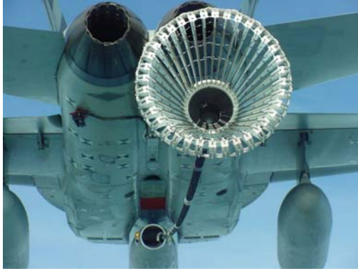
This is the pilot's view when docking with an F18 for refueling
